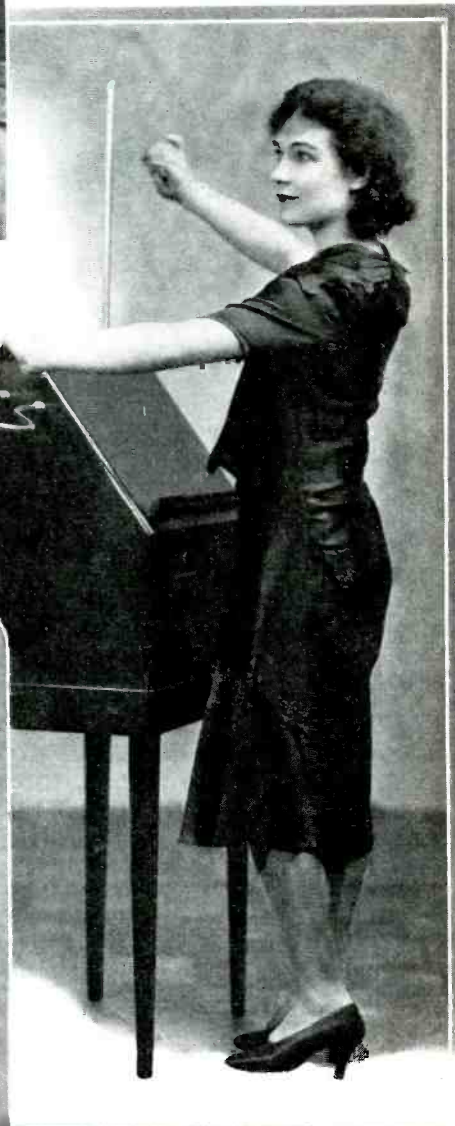
The Theremin, played by varying hand capacity, is already manufactured and sold by a large radio receiver manufacturer
