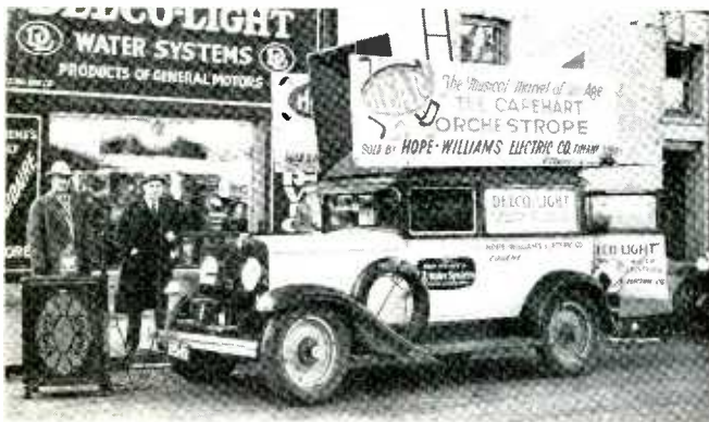
Any serviceman can rig up a motor-generator set in this manner, driving it from the car storage battery. Hope-Williams Electric, Eugene, Ore., demonstrates in a.c. "Orchestra" set.
